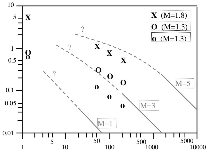
Figure 12 Far-field and projected near-field velocities for different magnitude events (from Jager and Ryder, 1999). Velocities for three of the modelled events have been superimposed on the original graph. The presence of the stope, and cases with a high stress-drop, lead to in-stope velocities associated with much larger magnitude events.
