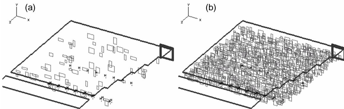
*Figure 13 Stope model with vertical fractures in the foot-wall of the stope. The fractures are rectangular with edge-lengths between 4 m and 14 m, and are in a band between 4 m and 18 m below the stope. (a) Fracture density of 0.01 (b) Fracture density of 0.1*
