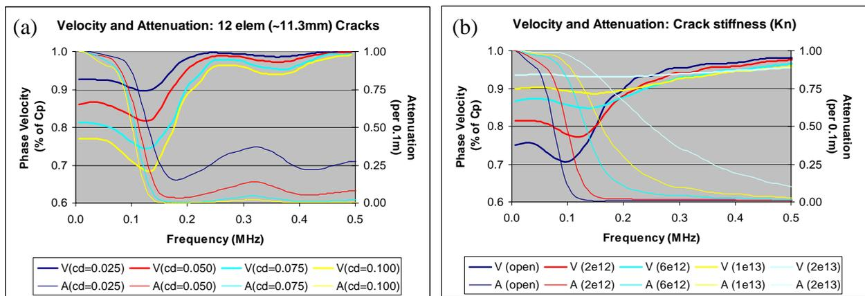
Figure 8 Phase velocity and attenuation spectra for crack distributions. (a) Distribution of 11.3 mm open cracks with a crack density of 0.025, 0.05, 0.075 and 0.1. (b) Distribution with crack lengths ranging from 7.3 mm to 19.3 mm, a crack density of 0.1, and varying fracture stiffness.
