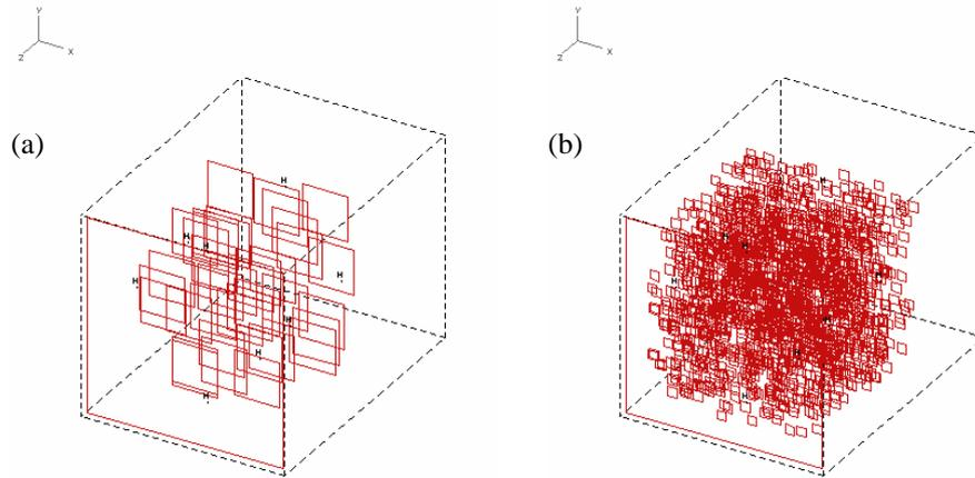
Figure 6 Crack assemblies with equal crack density ( $\varepsilon = 0.1$ ) (a) 38, 196.5 mm x 196.5 mm cracks (b) 6061, 36.5 mm x 36.5 mm cracks.
