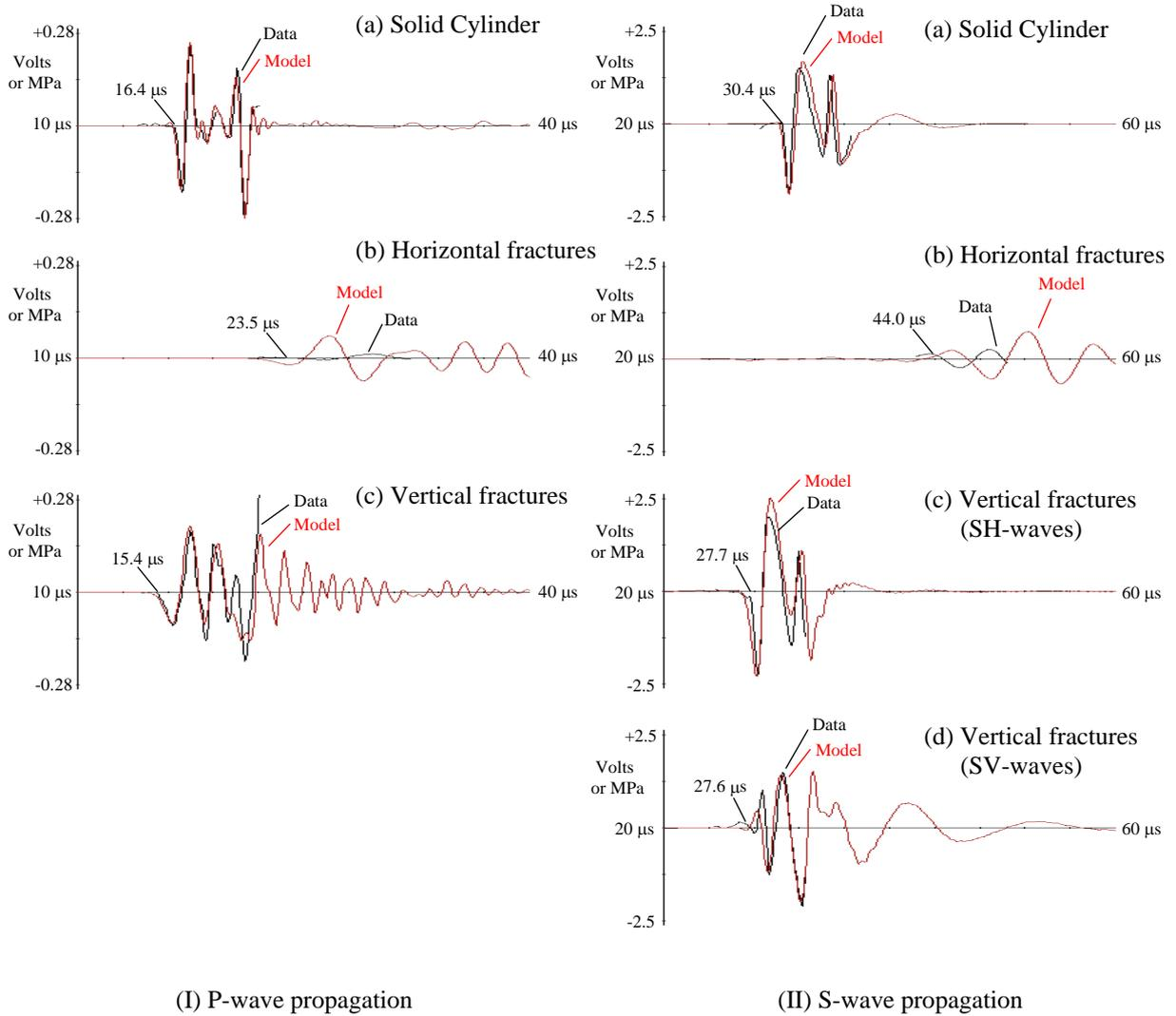
Figure 2 P- and S-wave comparisons of experimental and modelled waveforms for the different fracture orientations.
