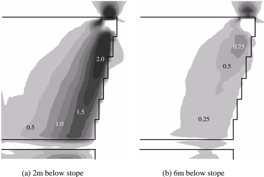
Figure 10 Maximum induced tensile stress (in MPa) for  $\sigma_{zz}$ . Plan sections are shown for two distances below the excavation, and indicate that horizontal tensile stress of up to 2 MPa is induced close to the surface, and that this falls off rapidly with distance from the surface.
