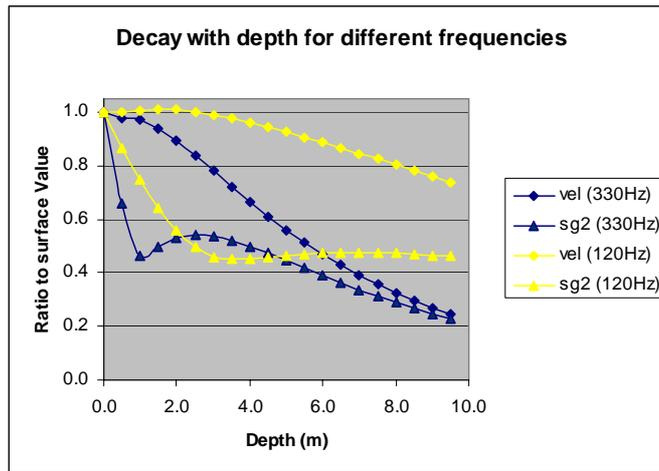
Figure 11 Decay rate of velocity and maximum tensile stress for different frequencies. (a) Peak frequency of 330 Hz ( $\lambda \approx 10$  m) (b) Peak frequency of 120 Hz ( $\lambda \approx 27$  m)
