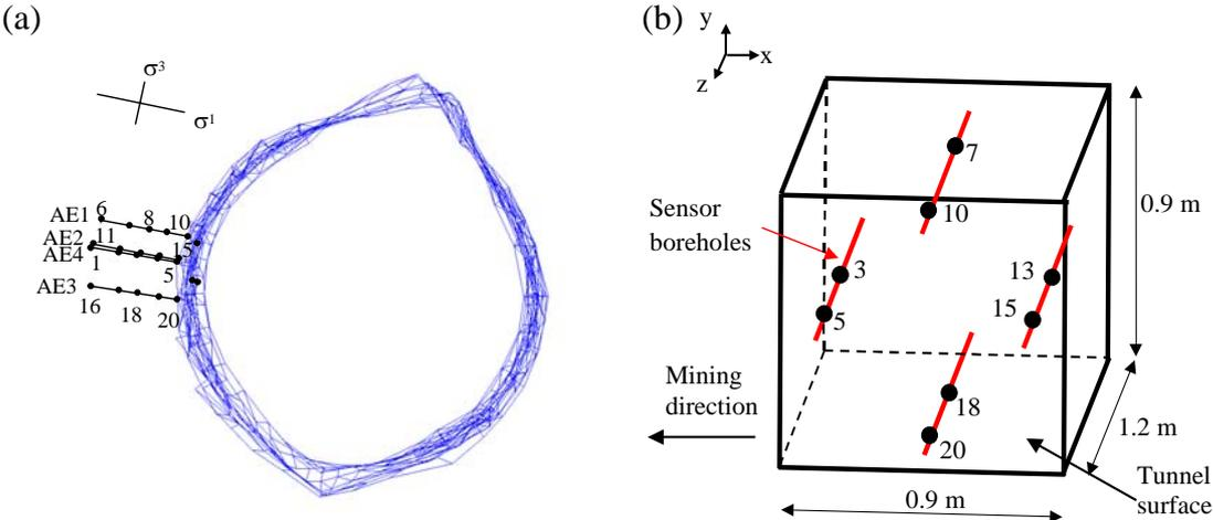
Figure 4 (a) Cross-sectional geometry of the acoustic array in the URL tunnel showing positions of boreholes AE1-AE4, and sensors 1-20. (b) Model geometry of a reduced 8x8 array, with boreholes rotated into a diamond pattern. The block indicates the model boundaries.
