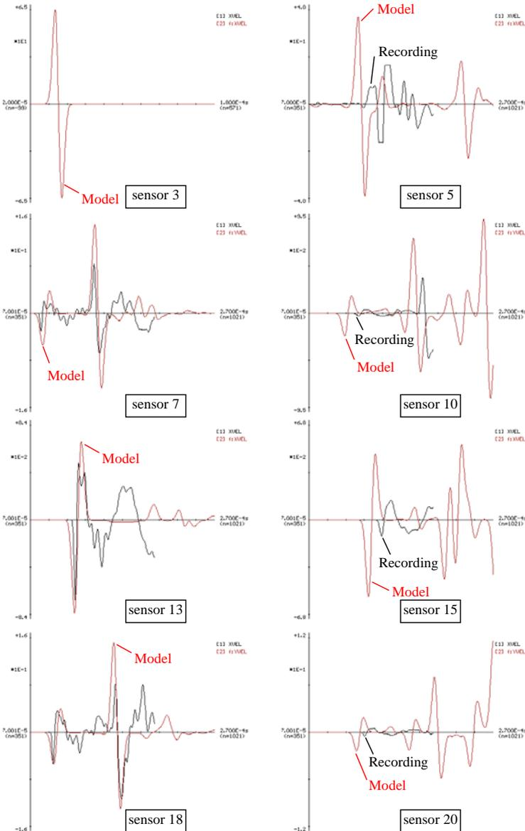
Figure 5 Elastic model (red line) compared to velocity scan AT01 (black line) for the source at sensor 3 – and receiver sensors 3, 5, 7, 10, 13, 15, 18, 20. Paths on the left were parallel to tunnel surface while those on the right were oblique to the tunnel surface.
