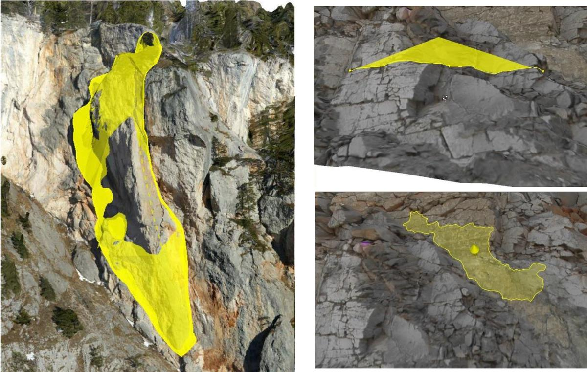
Figure 3: Quantification of a potentially detachable block with a volume of  $2.350 \text{ m}^3$  (left) and exemplary orientation measurements from a trace (top right) and from an area (bottom right).
