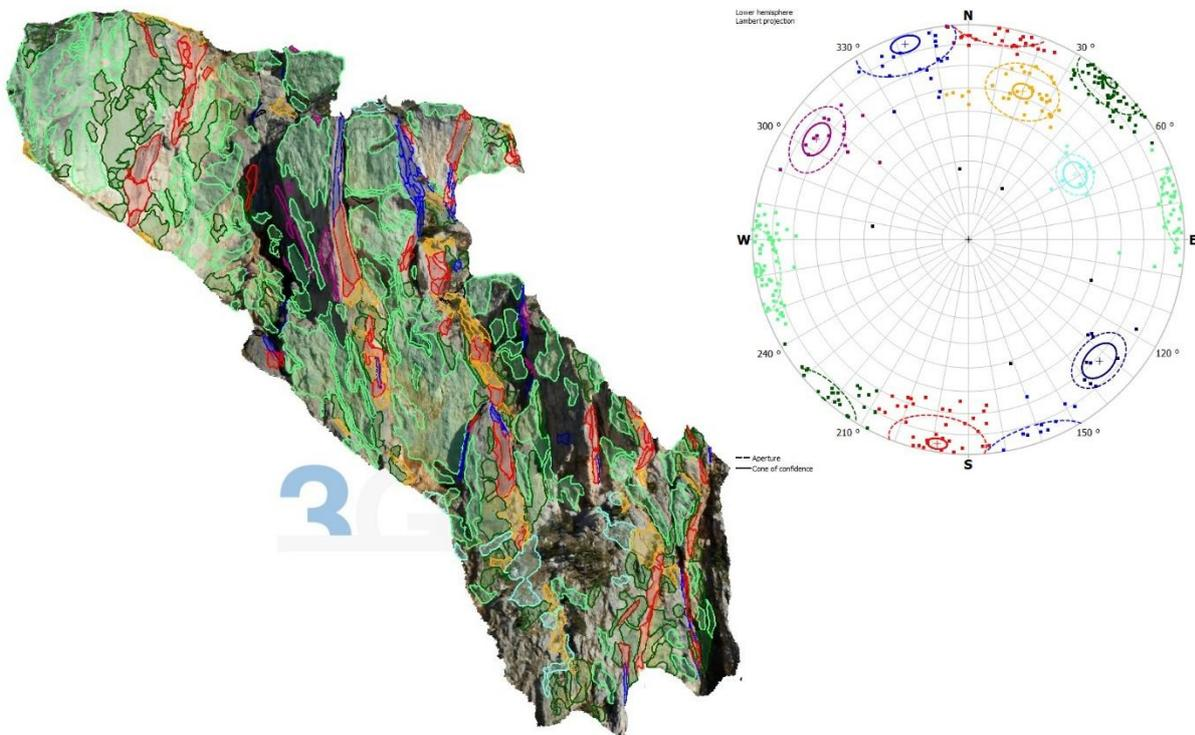
Figure 4: Automatic analysis of the hazardous area: identified structures (left) and discontinuity sets (right)
