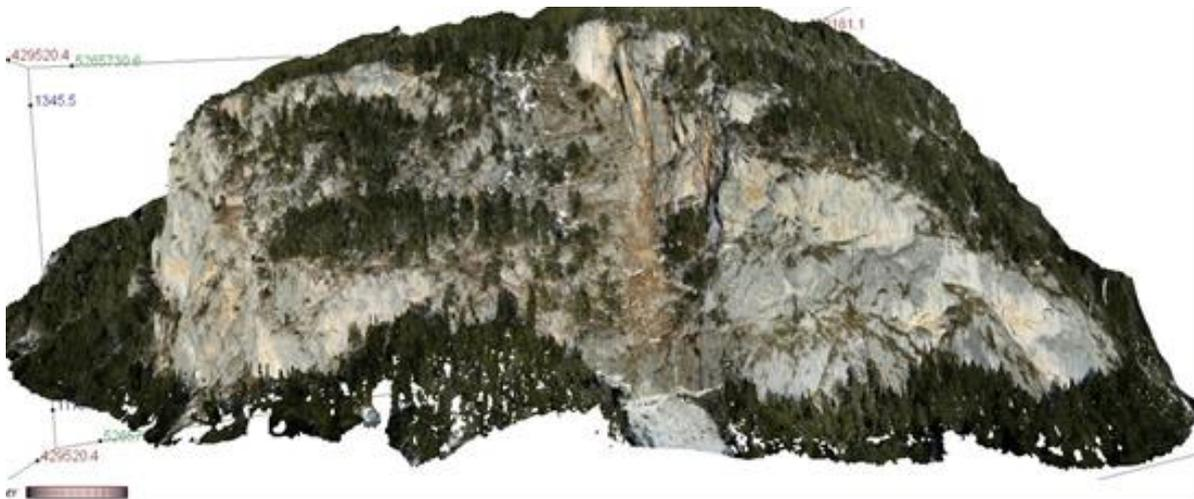
Figure 2: 3D model of a rock fall area in Austria captured close after an incident in the center part; overall size of the captured area: 750x250 m; vertical height: 200 m; flight time: 1 hour.
